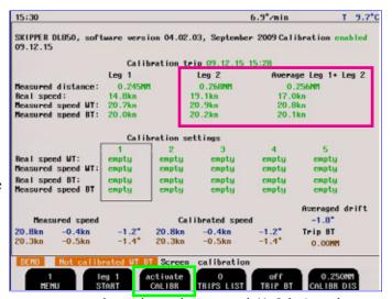
recommend a point at low speed (1-3 kn) and one at high speed (20 kn).
