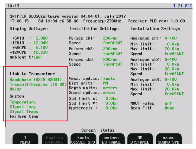
If it is at all possible to cycle through the screens and observe this information, several assumptions may be made regarding operation of the DL850 system. Although some of the subsystems necessary for this basic system operation may still suffer from minor or intermittent operation disorders, the fact that it is possible to select and observe this screen, indicate correct operation of the following DL850 subsystems:
