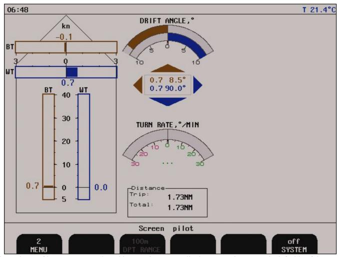
The various softkey menus are selected by pressing repeatedly the MENU button on the left side of the softkey menu. The number on the button indicates present active menu.
