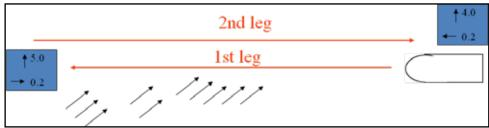
The 1st leg will show a different speed to the 2nd leg, however the direction changes in the second leg so that the average is correct.
