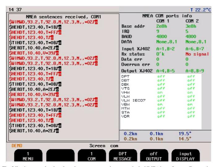
The following examples show how the system responds to errors in the NMEA input formats. Formats in yellow are rejected. See "NMEA Setup" on page 48 for more informations about accepted formats.
