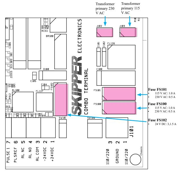
Fig. 4.1 Voltage selection connectors and fuses, Terminal Board.
