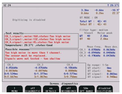
If the noise test fails in one channel only (on repeatable diagnostics tests)it is possible to temporarily disable the failing channel.
