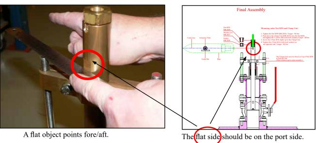
Fig 6.1 Sea valve alignment
