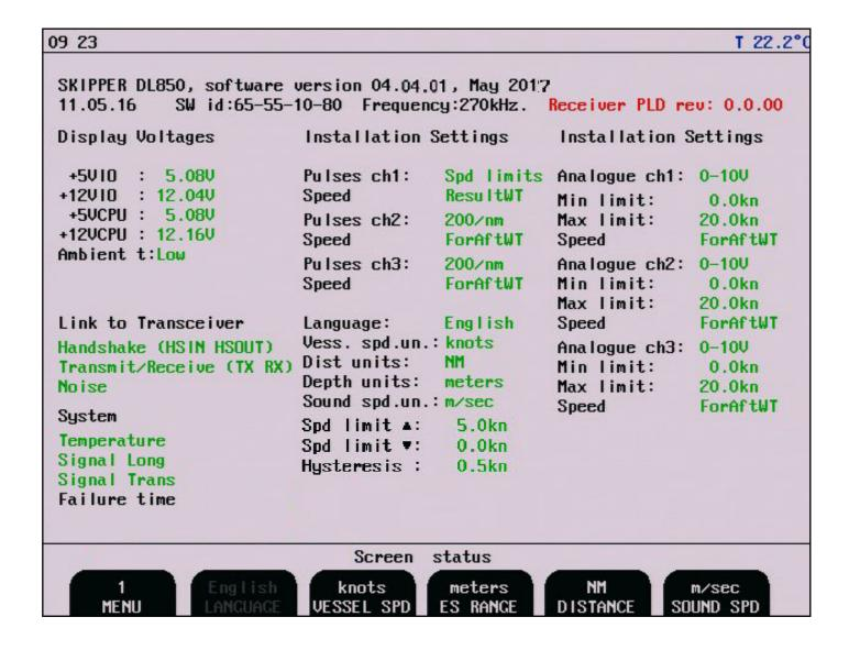
**Important note:** If, after power-up, on screen status, you see the following message "Receiver PLD rev: 0.0.00" in the upper right corner, this is an indication of old PLD in the transceiver unit. The unit will work, but is not optimized. Replace PLD with correct version, (1.0.00) or contact your local supplier for more information.
