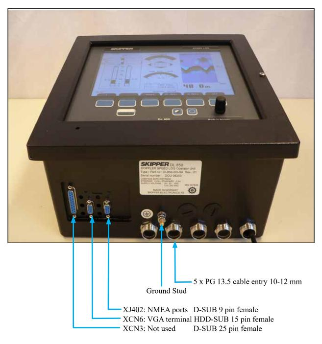
If required, the PG glands can be moved to other blinded holes. Extra holes are also available on back side of cabinet.
