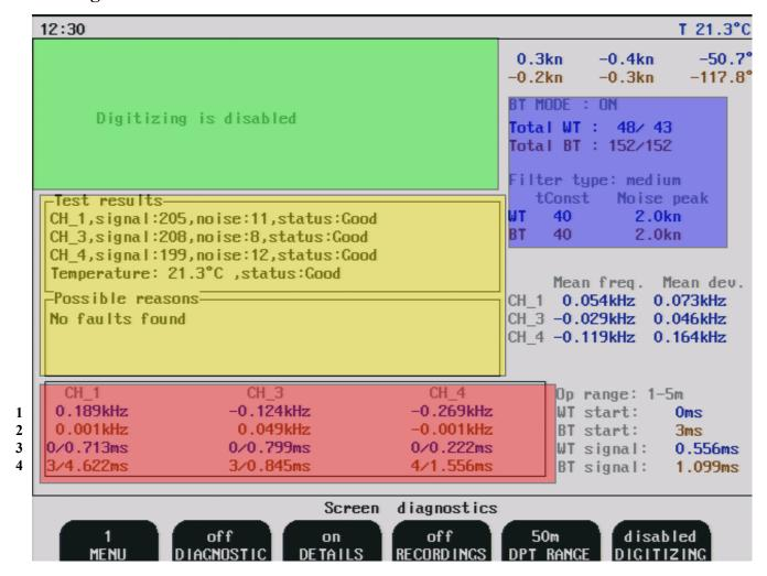
This diagnostic screen is used for self test and diagnostics and recordings of the system
