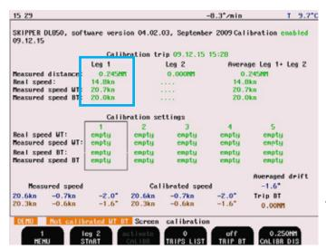
direction at the same speed. The results will show in the Leg 2 table. The average of the two legs will show in the final table. This is the correct calibration.
