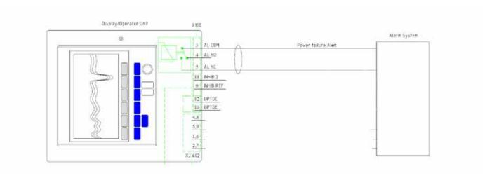
Fig. 4.7 Power failure connections
