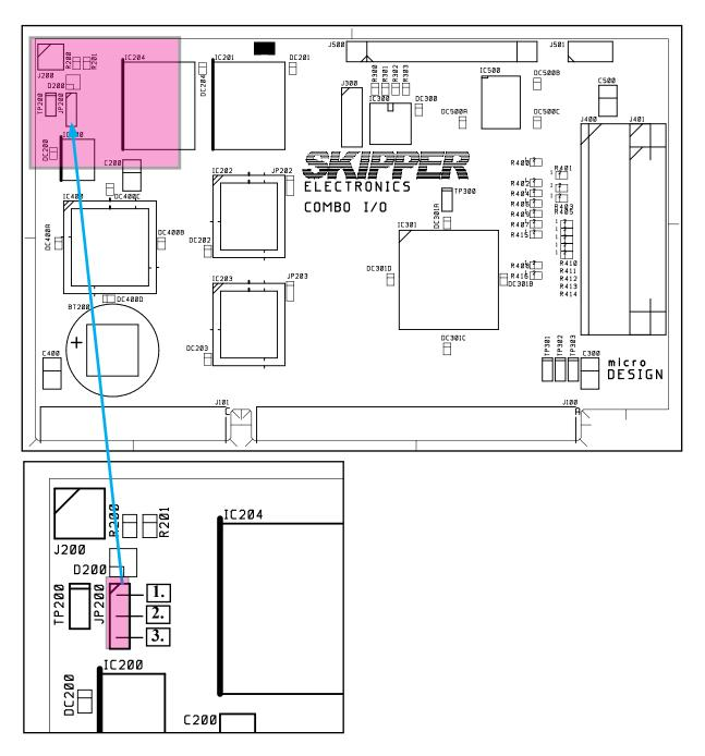
Fig. 4.2 Static Memory Battery Jumper, I/O Board.
