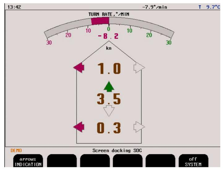
If bottom track is present, the docking screen will show measured longitudinal and transversal speed over ground (SOG) at fore and calculated speed at stern point. Speed indication may either be presented by values and arrows, or values and bars for directions.
