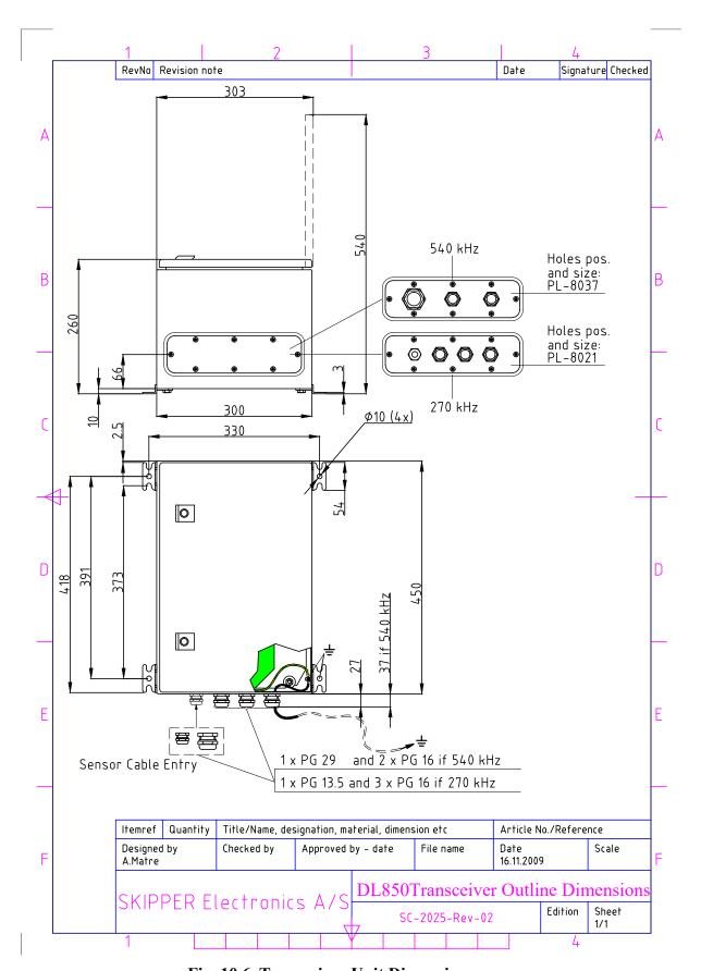
Fig. 10.6. Transceiver Unit Dimensions
