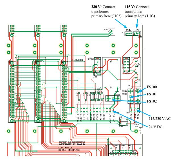
Fig. 10.8. 115/230 V selection on Transceiver unit backplane
