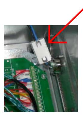
Fig. 10.5.1 Transceiver Unit EMC kit
