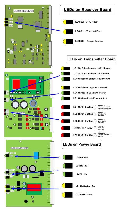
Fig. 10.2 LEDs on PCBs in Transceiver Unit
