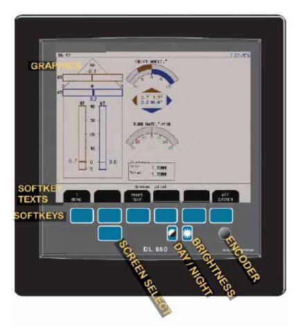
Fig. 1.1 Operator unit, panel layout.
